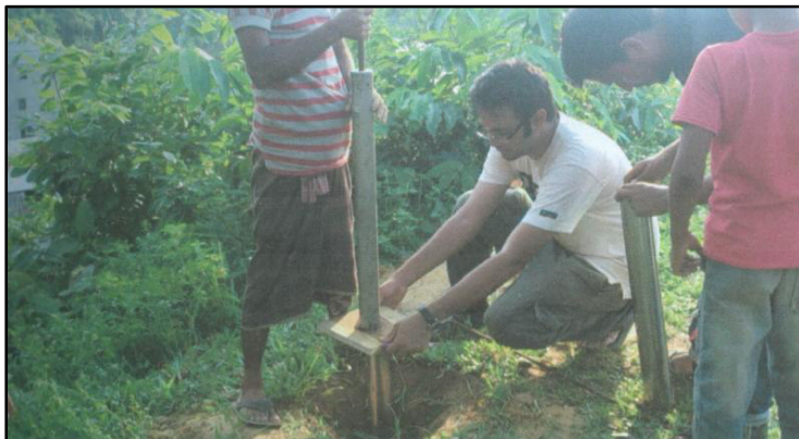
Figure 4.7: Inserting the Shelby tube deep into the ground by means of a 10 lb modified proctor hammer, blows were at a constant rate.
