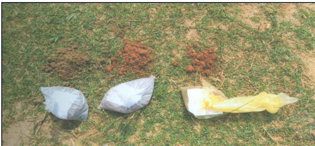
Figure 4.7: Collection of disturbed soil samples into separate polythene bags.
