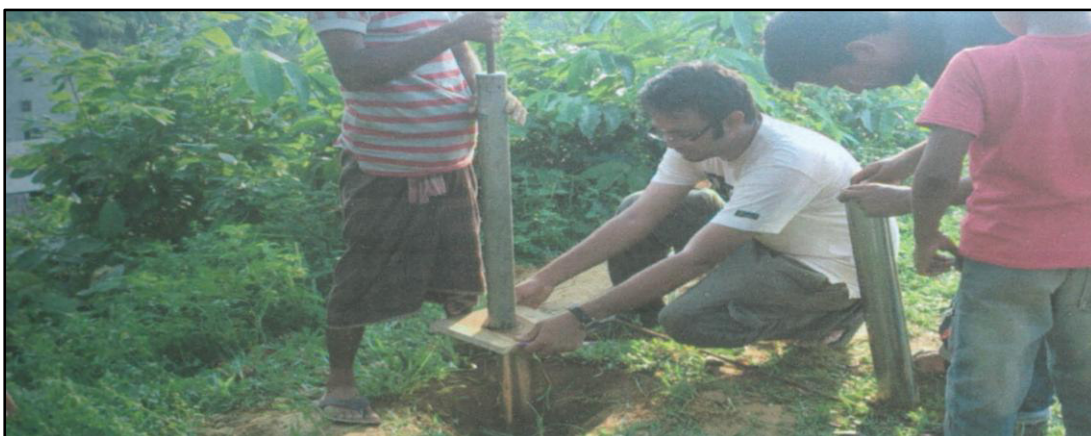
Figure 1.12: Inserting the Shelby tube deep into the ground by means of a 10 lb modified proctor hammer, blows were at a constant rate.
